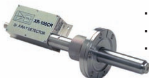
XR100CR fitted for vacuum applications
